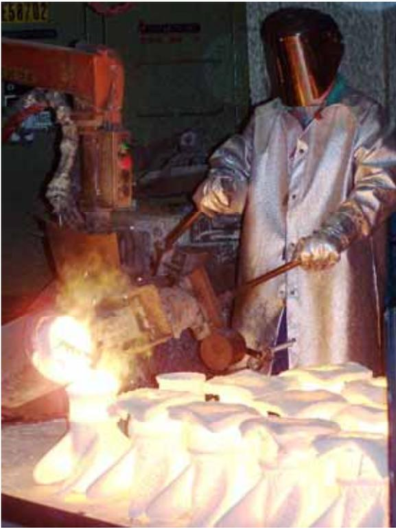
Furnace Operator Jerrred Nelson pours melted stainless steel into shells
