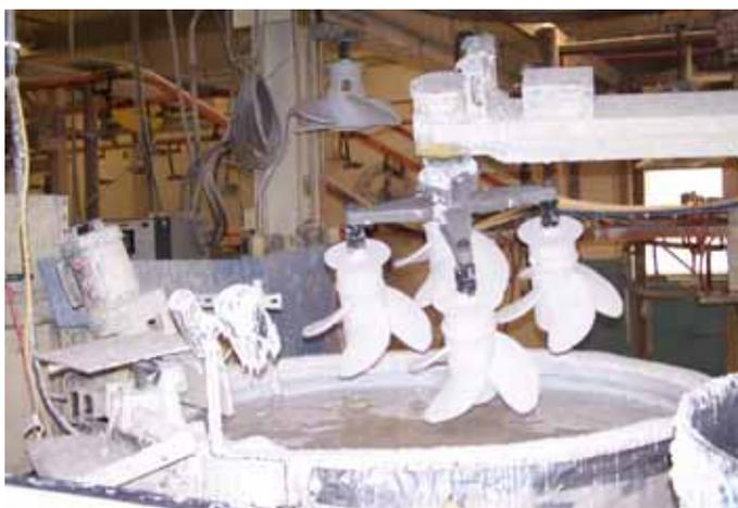
Wax patterns are dipped in ceramic 5 times to make a strong, thick shell
