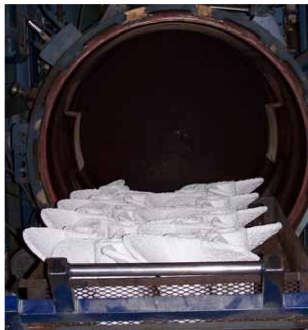
Wax is melted off by 180-degree steam in autoclave
