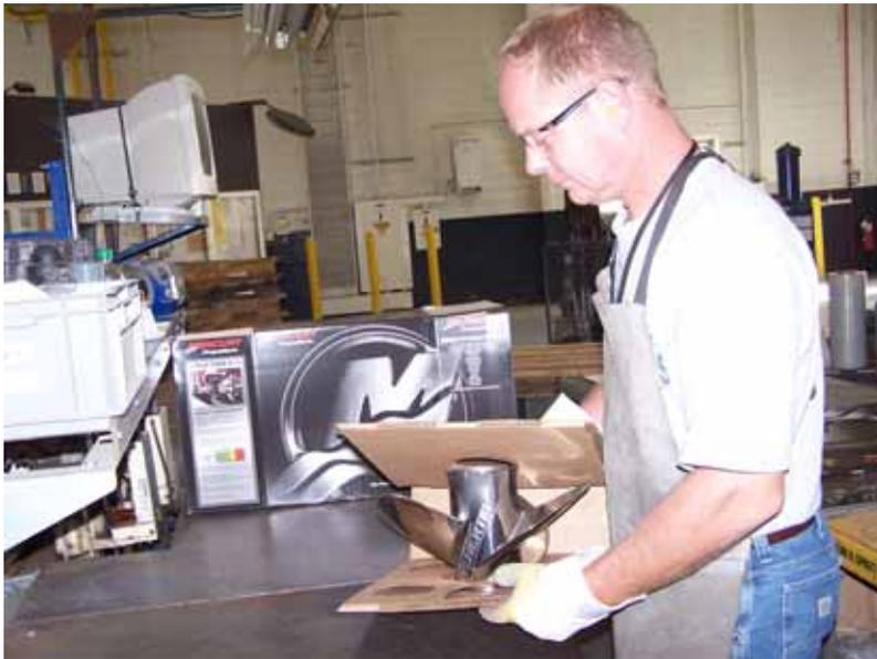
After the prop goes through surface refinery, Sam Thuerwachter boxes up a finished Enertia propeller
