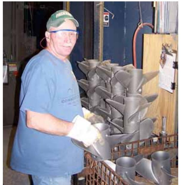
Cleaning cell operator Phil Gabatholer removes ceramic residue with a sandblaster
